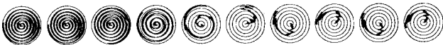
FIG. 2. Polar representation of the temporal evolution of the rotation angles for the different cylinders. The cylinders' positions are represented as circles. The distance from a point of a curve to the center of its circle represents the time.
